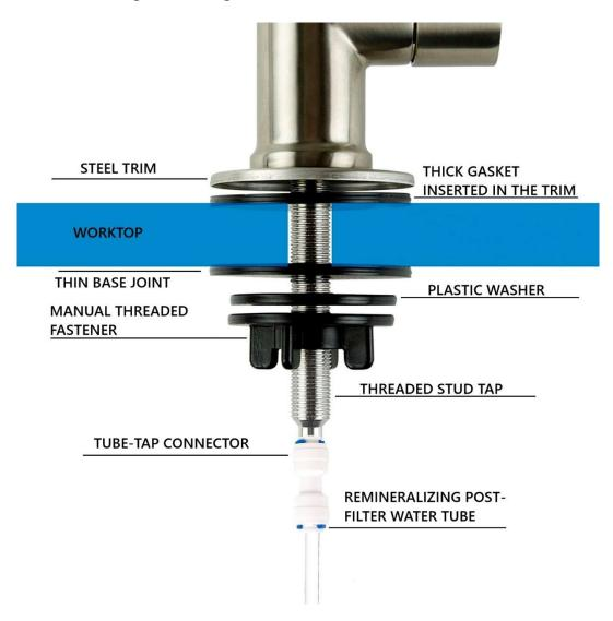
As shown in the diagram above, the faucet is equipped with a fastener, which does not require a tool to tighten it. The supplied link will be connected to the base stud. Once the tap is installed, the cap of the yellow remineralizing post-filter will be removed, the pipe will be connected, the necessary section will be measured and cut to insert it into the tap connector.
