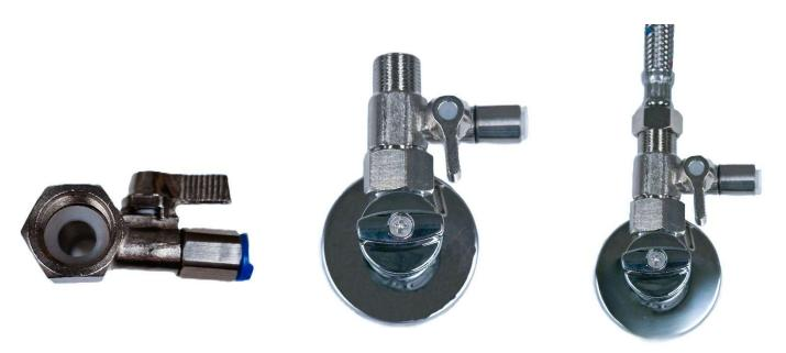
To connect the supply pipe to the equipment, we remove the blue clip from the key connector, insert the supplied pipe all the way up, place the blue clip in its original position.
