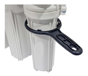
Once the first 3 filters have been installed, the membrane is installed. To do this, the blue clip will be removed from the elbow of the membrane holder and, as indicated in the diagram, which appears at the bottom of this page, the elbow tube will be removed. This operation can be performed with the help of a lever, without damaging the elbow.
